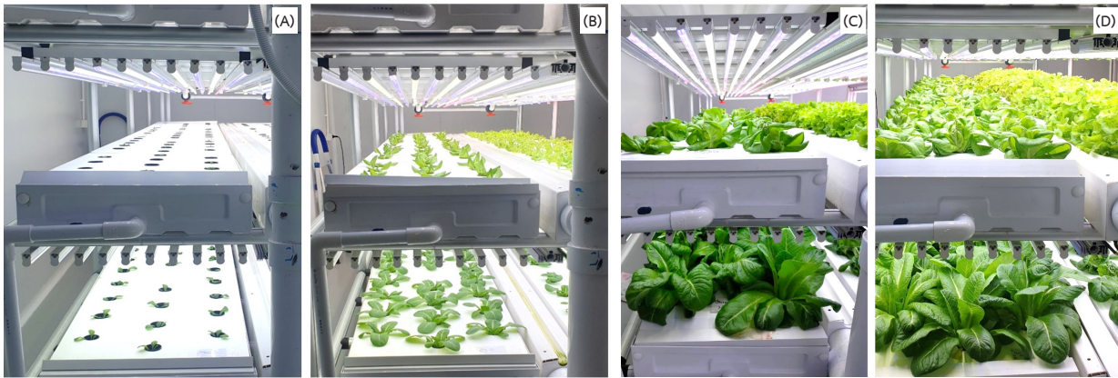
Figure 1 Development of lettuce in a plant factory with artificial lighting (PFAL) at 1 (A), 2 (B), 3 (C), and 4 (D) weeks after transplanting
