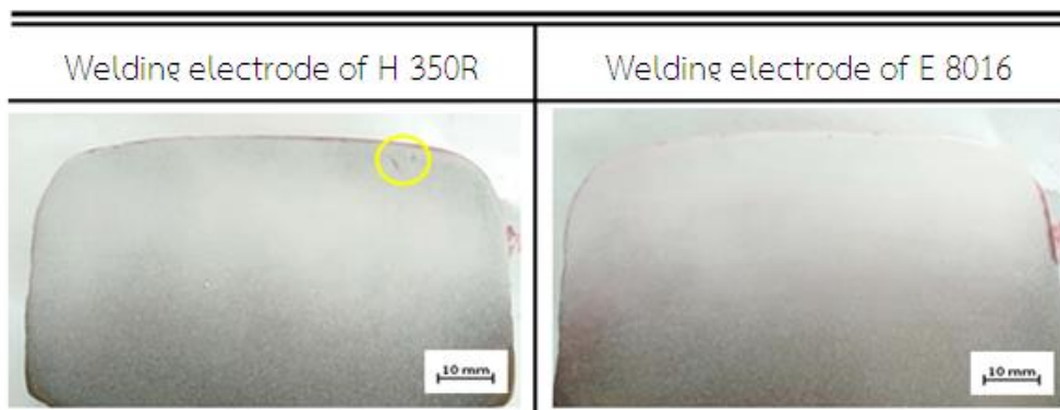
Figure 4 Examine the cross-section surface with penetrant testing (PT)
