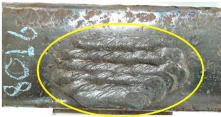
Figure 1 Surface hard-facing welding of 100 pound/yard railway
