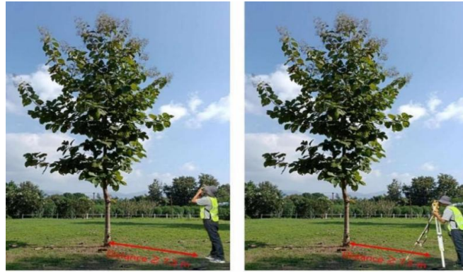
Figure 2 illustrates the field setups: Laser Rangefinder (left), and Total Station (right).
