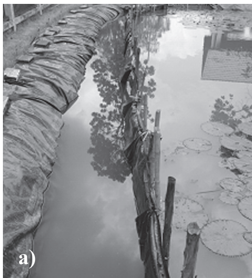
Figure 1. a) Polyethylene flume; b) Pilsbryoconcha exilis compressa
