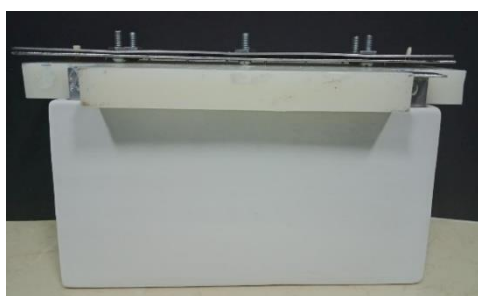
Figure 1 (Left) Coating chamber and (Right) electrodes inside the chamber
