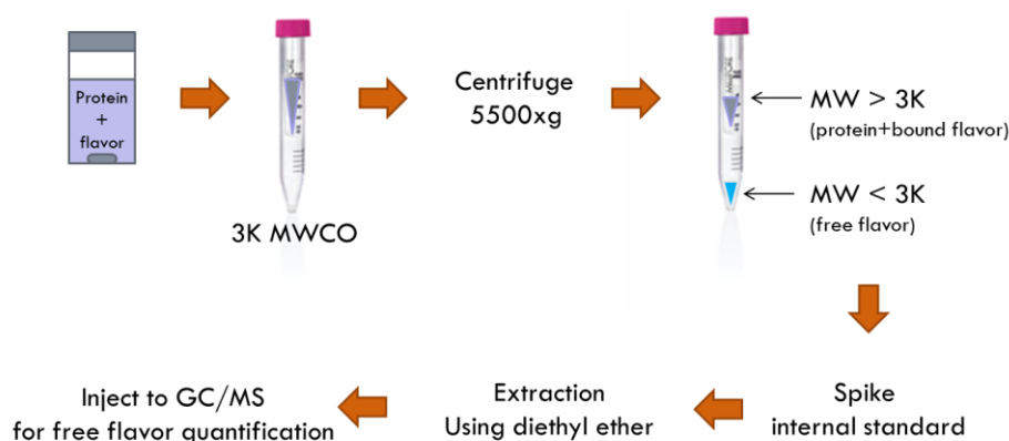
Figure 2 Flow diagram for isolation and quantification of free flavor compounds [17]
