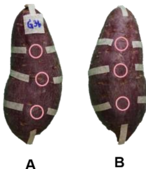
Figure 1 Spectral acquisition: 6 points per tuber, (A) front and (B) back views of sample
