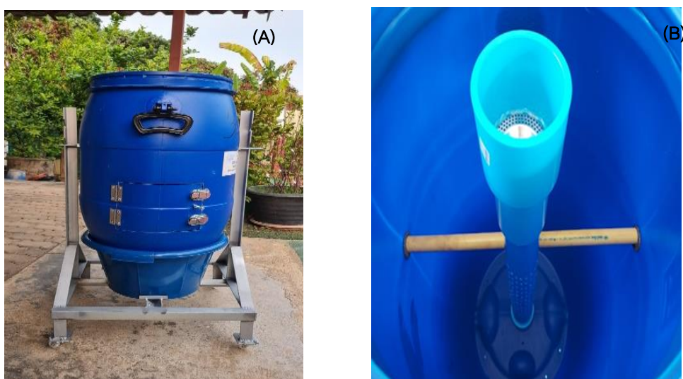
Figure 1 (A) External characteristic of bin and (B) Core ventilation pipe in compost bin
