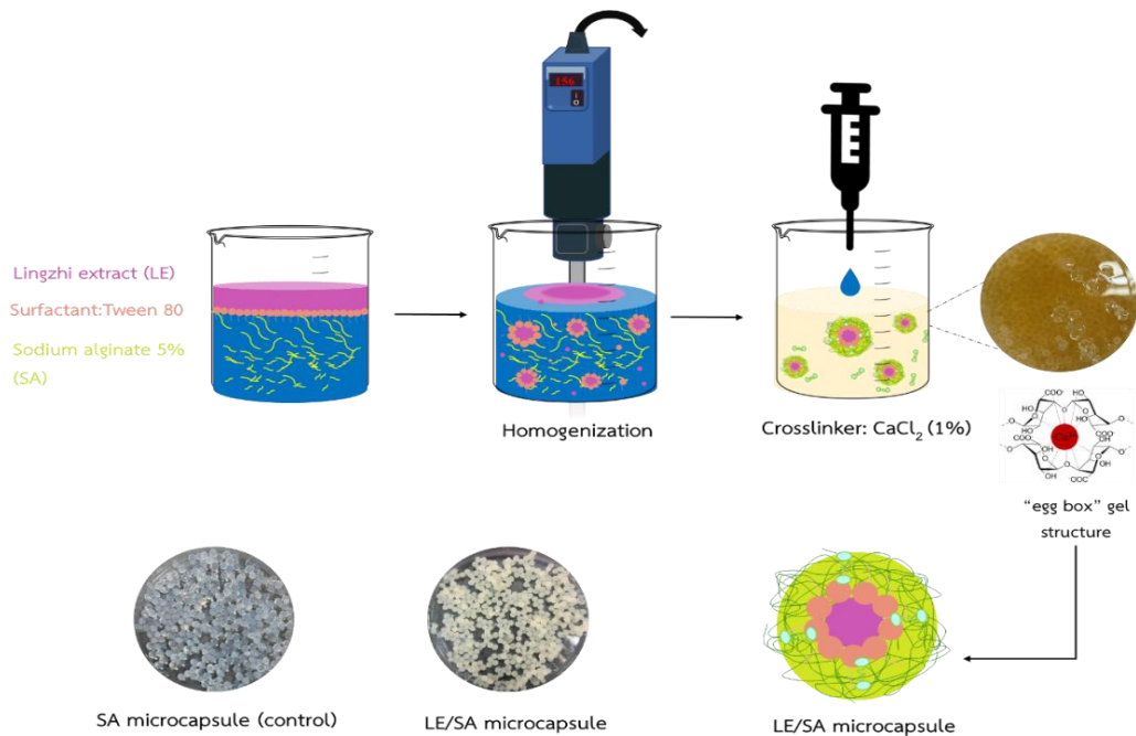
Figure 1 Schematic for step of preparation of LE/SA microcapsule
