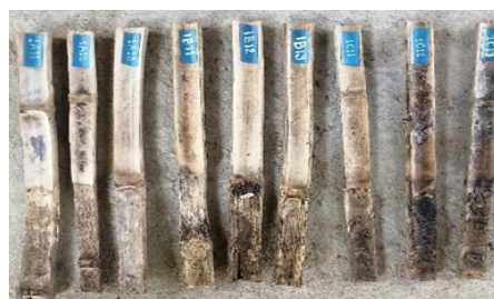
(b) Bamboo specimens after testing
