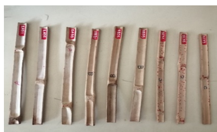
(b) Bamboo specimens after testing
