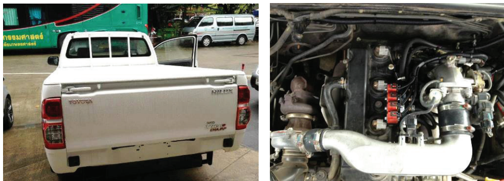
Figure 1 (left) Toyota Hilux Vigo and (right) Diesel-Dual-Fuel engine
