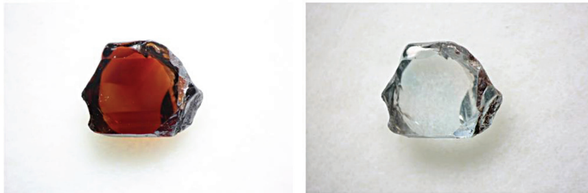
Figure 12 The color changing of reddish brown zircon from Ratanakiri, Cambodia between before (left) and after (right) heat treated in the SiC crucible model with reduction environment for 60 minutes with power 800 watts, average temperature 900 °C.
