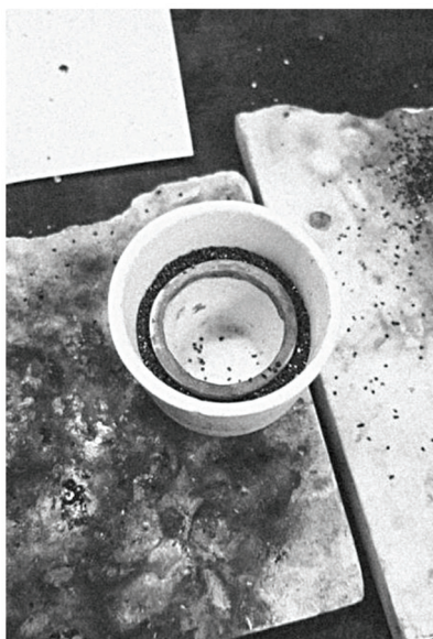
Figure 2 Model of crucibles for the grain-type silicon carbide experiment.
