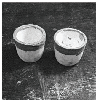
Figure 1 Model of crucibles for powder-type silicon carbide experiment.
