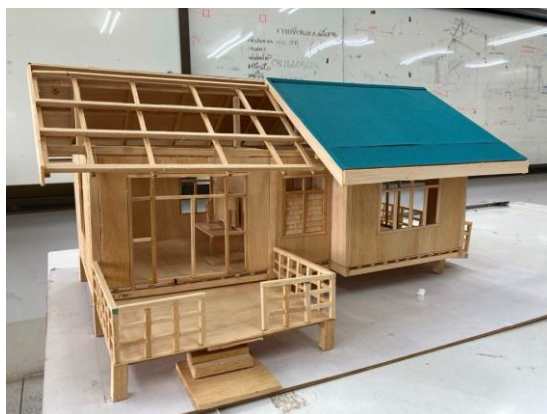
Figure 8. Structure model from construction drawings
