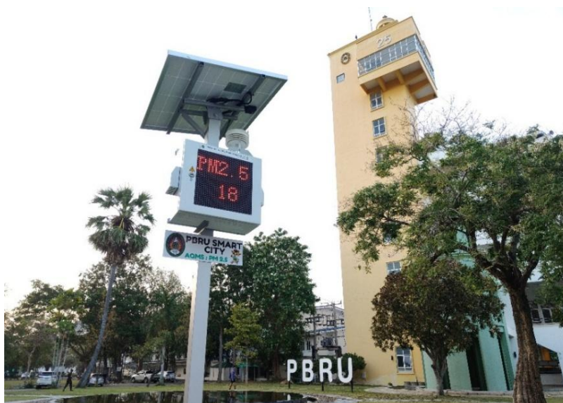
Figure 4. Air Quality Monitoring Station
