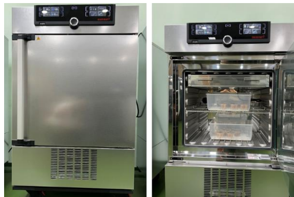
Figure 1. Khanom La samples were placed in an accelerated chamber to maintain storage temperatures at 25°C and 35°C for 35 days.
