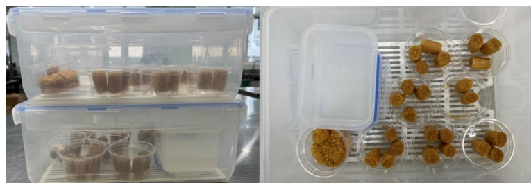
Figure 2. Khanom La samples were placed in airtight containers at ambient temperature to control water activity for obtaining the sorption isotherm curve of Khanom La.
