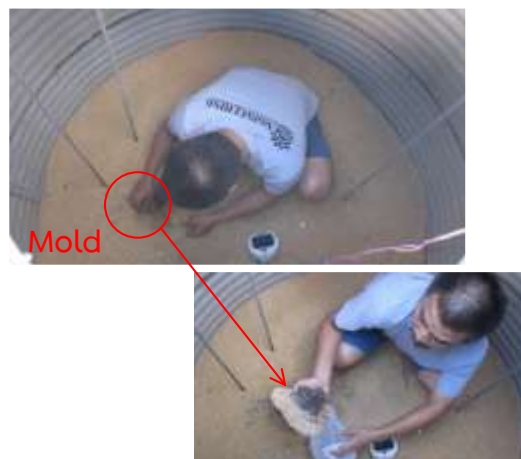
Figure 8 Unexpected mold at the top of grain surface in the silo with simulated insect infestation.
