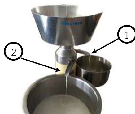
Figure 1 Disc and bowl centrifugal separator. 1. Coconut cream, 2. Coconut skimmed milk
