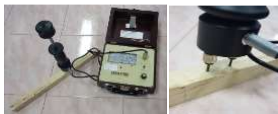
Figure 3 Measurement of moisture content using pin moisture meter
