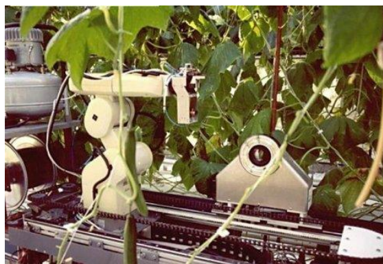
Figure 3 Cucumber harvesting robot.
