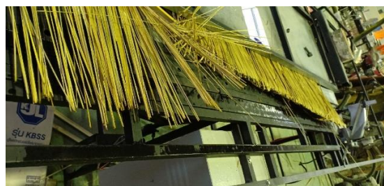
Figure 19 Fail of wood stick gripping mechanism.
