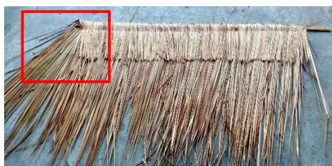
Figure 15 Wrong sewing at the first of operation.
