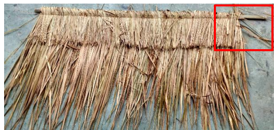
Figure 17 Incomplete sewing at the end of operation.
