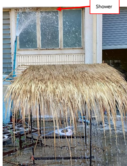
Figure 10 Leakage test by shower.
