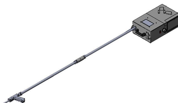
Figure 2 Drafts of portable commercial cane sugar analyzer by near infrared technique.
