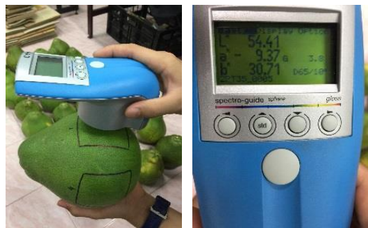
Figure 3 VIS spectral acquisition of pomelo in reflectance mode using spectrophotometer (spectro-guide sphere gloss BYK-Gardner GmbH, Germany).
