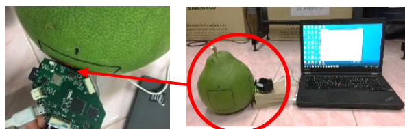
Figure 2 NIR spectral acquisition of pomelo in reflectance mode using NIRscan Nano EVM (Texas Instruments, Dallas, Texas, USA).
