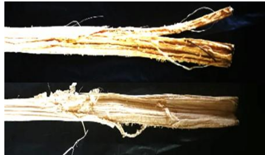
Figure 8 Example of damaged banana rope.
