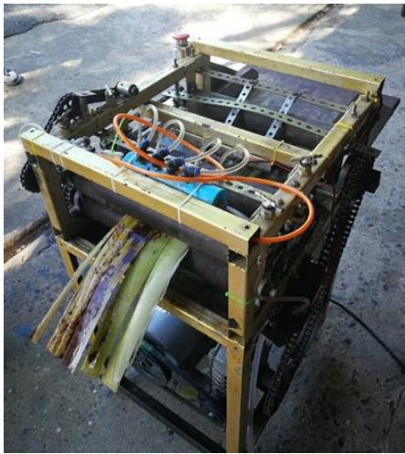
Figure 6 The completed banana leaf sheath preparing machine.
