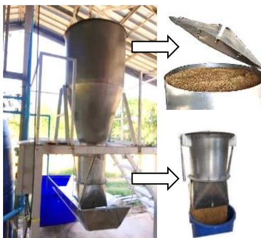
Figure 3. The composition of paddy tank.
