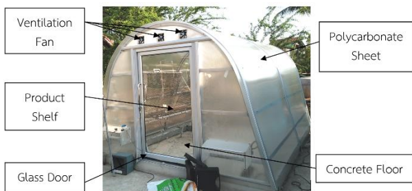
Figure 1 The solar greenhouse dryer.
