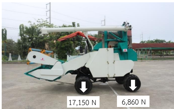
Figure 5 The difference forces acted on the wheels at the front and rear axle.
