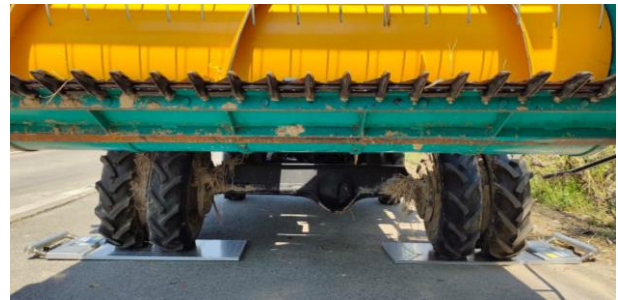
Figure 2 Weigh Rice combine harvester.
