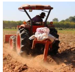
Figure 3. Preliminary test of weighting at the digger disc position.
