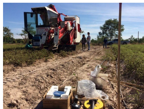
Figure 13 The imported peanut combined harvester.
