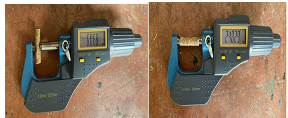
Figure 9 Measurement of dimension of pellets of cassava stems.
