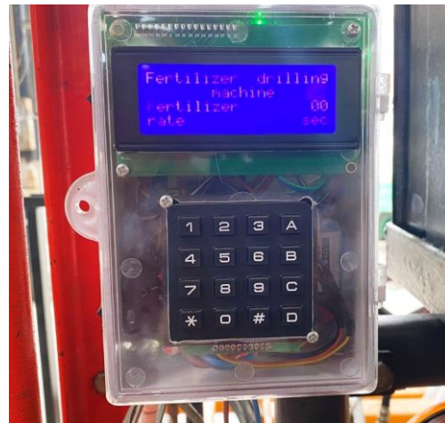
Figure 5 Inputting fertilizer rate via keypad on control panel.
