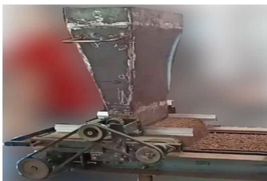
Figure 4 Soil sprinkling set.
