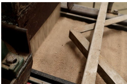
Figure 6 Sand sprinkling set.
