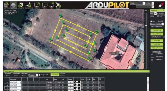
Figure 7 Pattern for testing the distance of start-stop.
