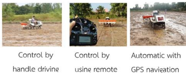
Figure 3 pattern for driving a vehicle.
