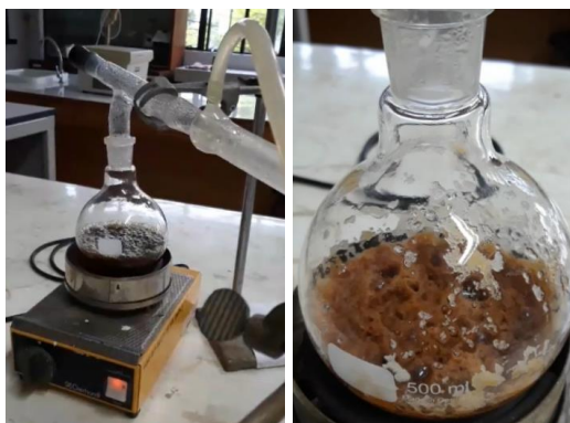
Figure 1 Distillation of fish sauce using a standard distillation set.
