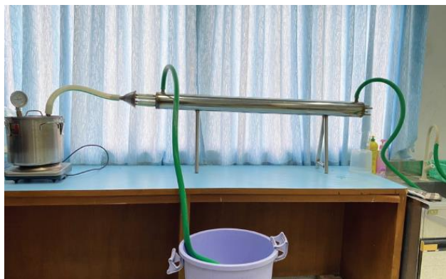
Figure 3 Distillation of fish sauce using a fish sauce distillation machine.
