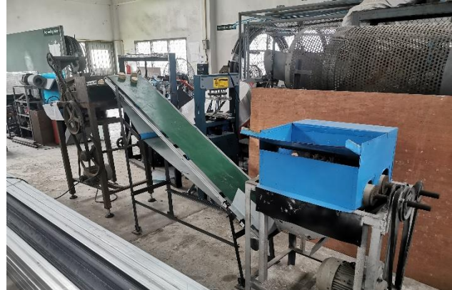
Figure 8 Cassava cubes cutting system.
