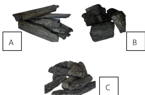
Figure 3 Characteristics of charcoal produced using 3-step charcoal kiln (A) Bamboo charcoal (B) Longan wood charcoal (C) Corn cob charcoal.
