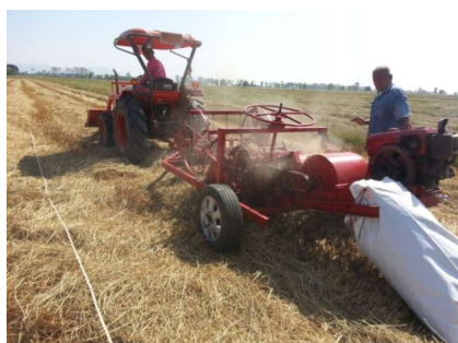
Figure 2 Measurement of the amount of straw and stubble cutting at different rotational speeds of the suction screw unit.
