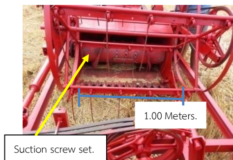
Figure 3 Suction screw set for transporting straw and stubble to be cut and chopped.
