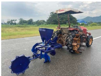
Figure 3 Tractor-mounted cassava weeding machine.
