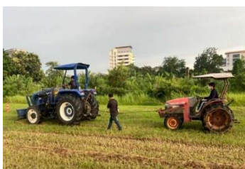
Figure 6 Field measurement of tractor drawbar power.
