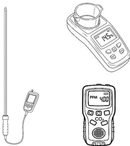
Figure 1 Example of a handheld grain temperature probe (left), moisture tester (upper-right) and carbon dioxide monitor (lower-right).
