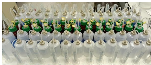
Figure 7 Experimental setup for assessing biological methane potential (BMP).
