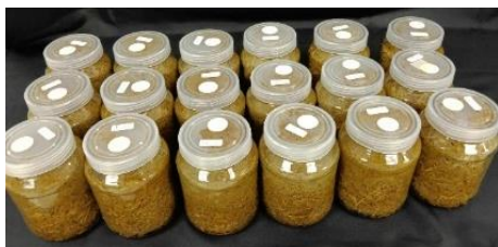
Figure 5 Experimental setup for pretreating sugarcane leaves with spent oyster mushroom substrate under aerated conditions.
