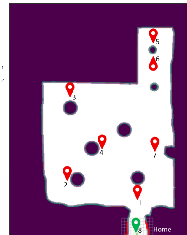
Figure 6 Simulation in RViz environment layout illustrating the configuration of static obstacles and the eight designated target waypoints used in the experimental
