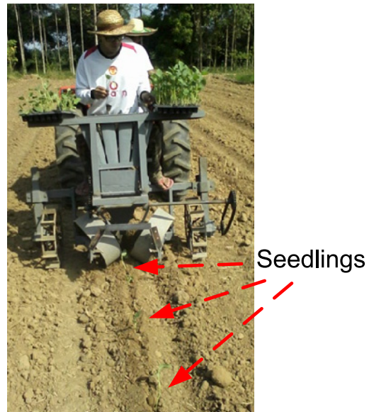
Figure 4 The mechanical transplanter during the performance tests.
