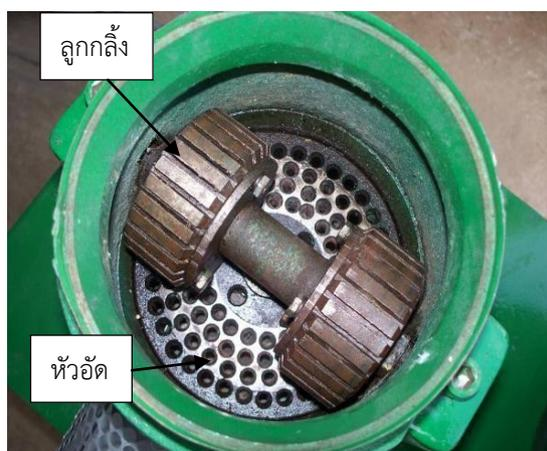
Figure 1 Flat die machine used in this study.
