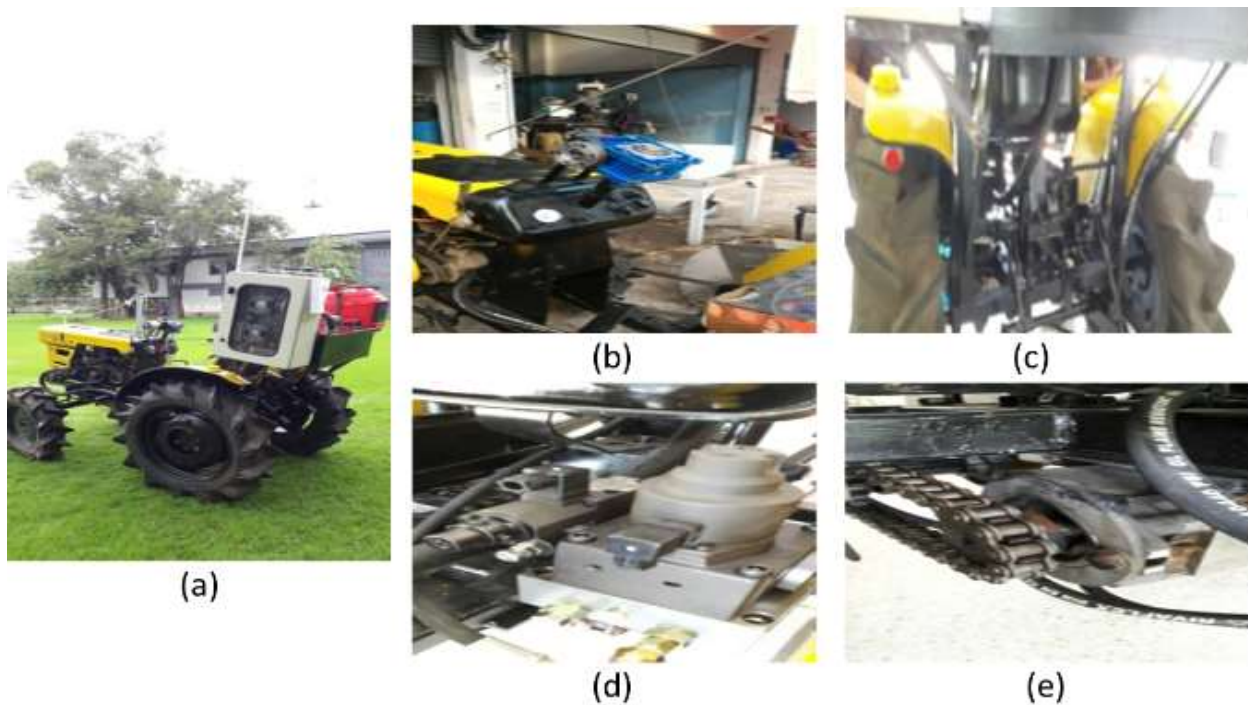
Figure 10 Specifications of the sensors. (a) Autonomous tractor based on GPS guidance; (b) Gear reducer for steering; (c) 3 point hitch for drawbar; (d) Proportional electro-hydraulic pressure control valve; (e) Hydraulic motor.
