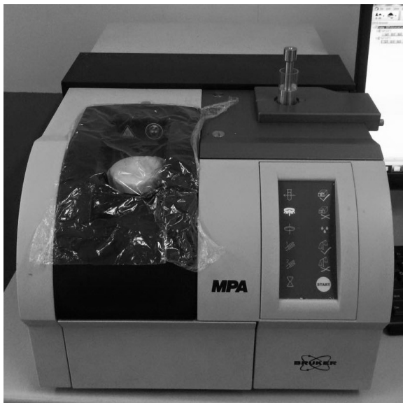
Figure 1 Spectra measurement of milk by FT-NIR spectrometer.
