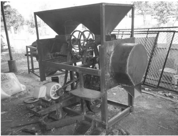
Figure 4 Components of develop two pelleting die organic fertilizer compression machine.
