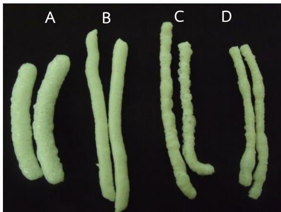
Figure 4 Loose-fill foam by extrusion process (A) PBS, (B) TPS20, (C) TPS30 and (D) TPS40.
