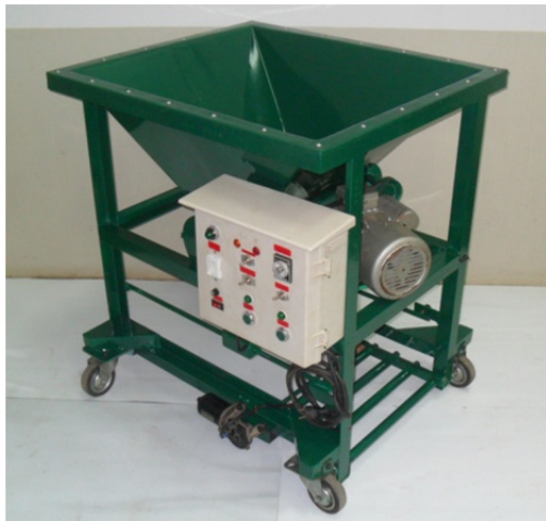
Figure 3 The soil packing machine for pre-transplanting para rubber bags, Model 2.
