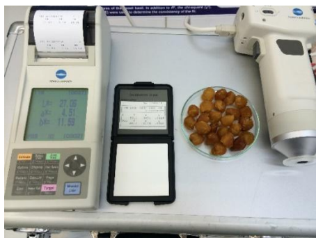
Figure 2. Photography of CR-400 chroma meter (Konica Minolta; Japan).
