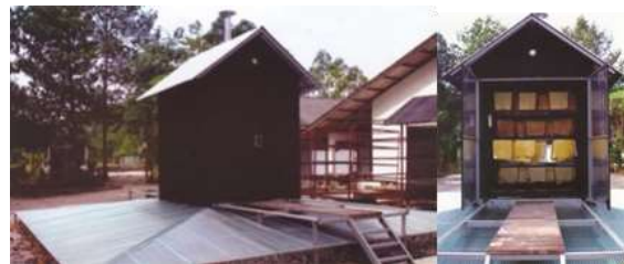
Figure 4 Rubber sheet greenhouse dryer of Department of Agriculture.
