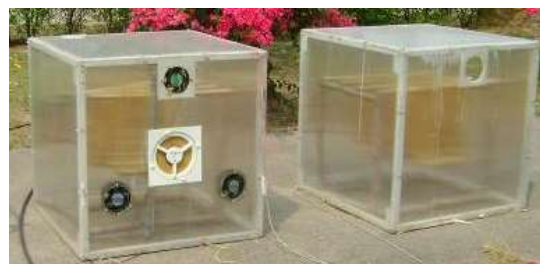
Figure 5 Rubber sheet drying test in the solar greenhouse dryer model controlled and uncontrolled temperature.
