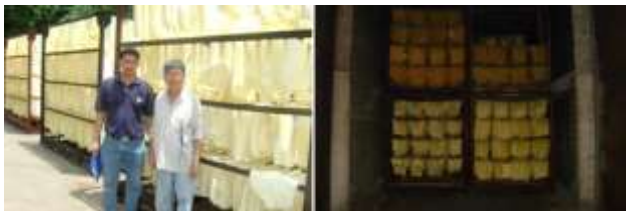
Figure 2 Rubber sheet drying method of commercial scale.
