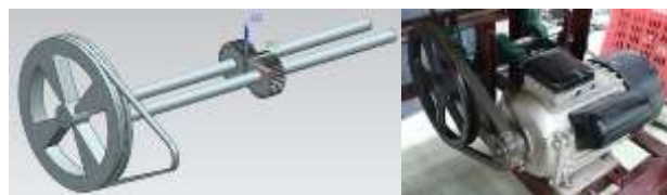
Figure 2 Reverse gear assembly drawing and details of a sapodilla sorting machine.
