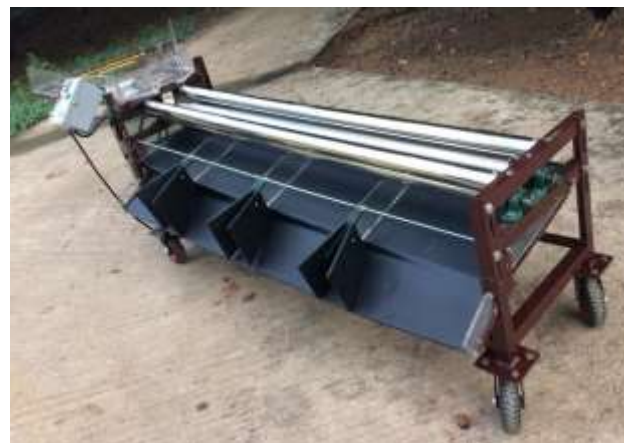
Figure 3 The sapodilla sizing machine using expanding rollers, Model 2.
